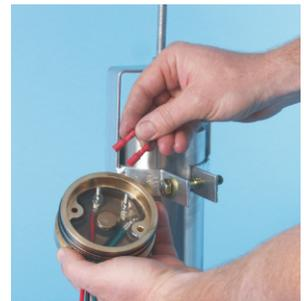
4. Place the push plate across the two motor nuts with center hole facing up.
