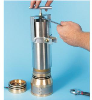
7. Remove the stainless steel housing and push plate.
