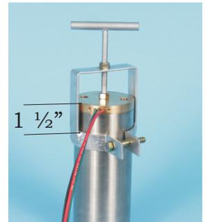
2. Hold the pump with one hand while turning the top nut clockwise, using a 9/16" wrench, until the end cap is completely out of the housing.
